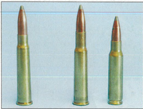
The U.S. Army semi-copied the .303 British (left) when developing the .30-40 Krag (center), but gave the .30-40 a much longer neck. However, in 1920, the very short-necked .300 Savage appeared (right), which almost matches the powder capacity of the .303 and .30-40.
